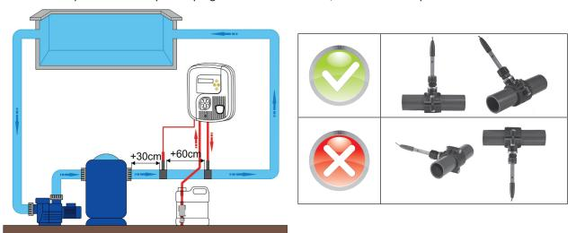
• The liquid chlorine injection point must be positioned before a pH corrector injection point and after the heating system.
