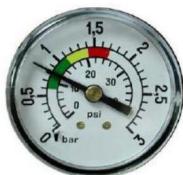
0.8 kg/cm 2 - 11.4 PSI: initial pressure filter at the start of the filter cycle
