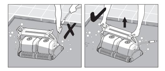
Using the floating cable, bring the Pool Cleaner to the pool's edge. Using the handle remove the Pool Cleaner from the pool.
