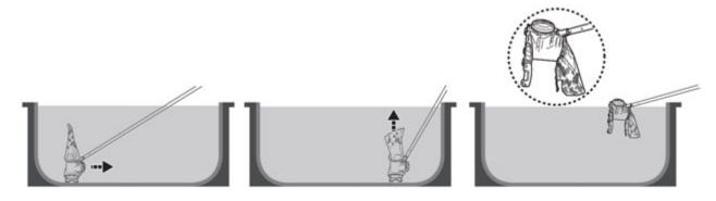
Once the pool vacuum is out of the water, the impeller will cease to spin within 2-3 seconds. The LED light will turn blue. When battery level is running low, blue light will flash.
