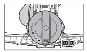
2. Align and attach the charging plug to the charging port. **WARNING!** Be sure not to invert the charging plug and ensure both the charging plug and charging port are clean and dry before charging them. TIPS: Use cotton bud to dry the charging port and pins. Plug the charging cable of the external adaptor into the charging plug.
