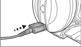
3. Connect the external adaptor to the power source. The indicator light on the external adaptor will turn red when the vacuum is charging and green when it is fully charged. Charge it for 5-6 hours for best performance.
