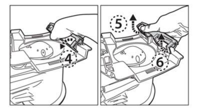
Before detaching the damaged front wheels, you will need to detach the frame first.
