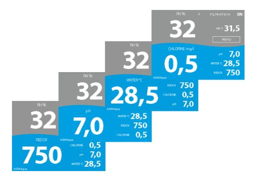
Lower part of the display can show informations about water temperature, pH, Redox or Chlorine
