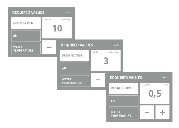
Setup of required values for SANOSIL, DOSE, CHLORINE, pH and water temperature
